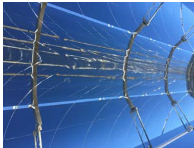
► Eucomsa has manufactured spare parts for the parabolic trough collectors of the Xina Solar One solar plant in South Africa.
