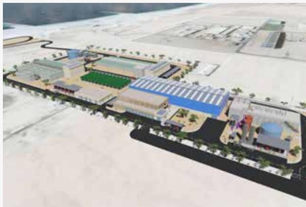
► Desalination plant in Salalah, Oman, which will operate with reverse osmosis technology and will have a capacity of 114,000 m<sup>3</sup>/day.
