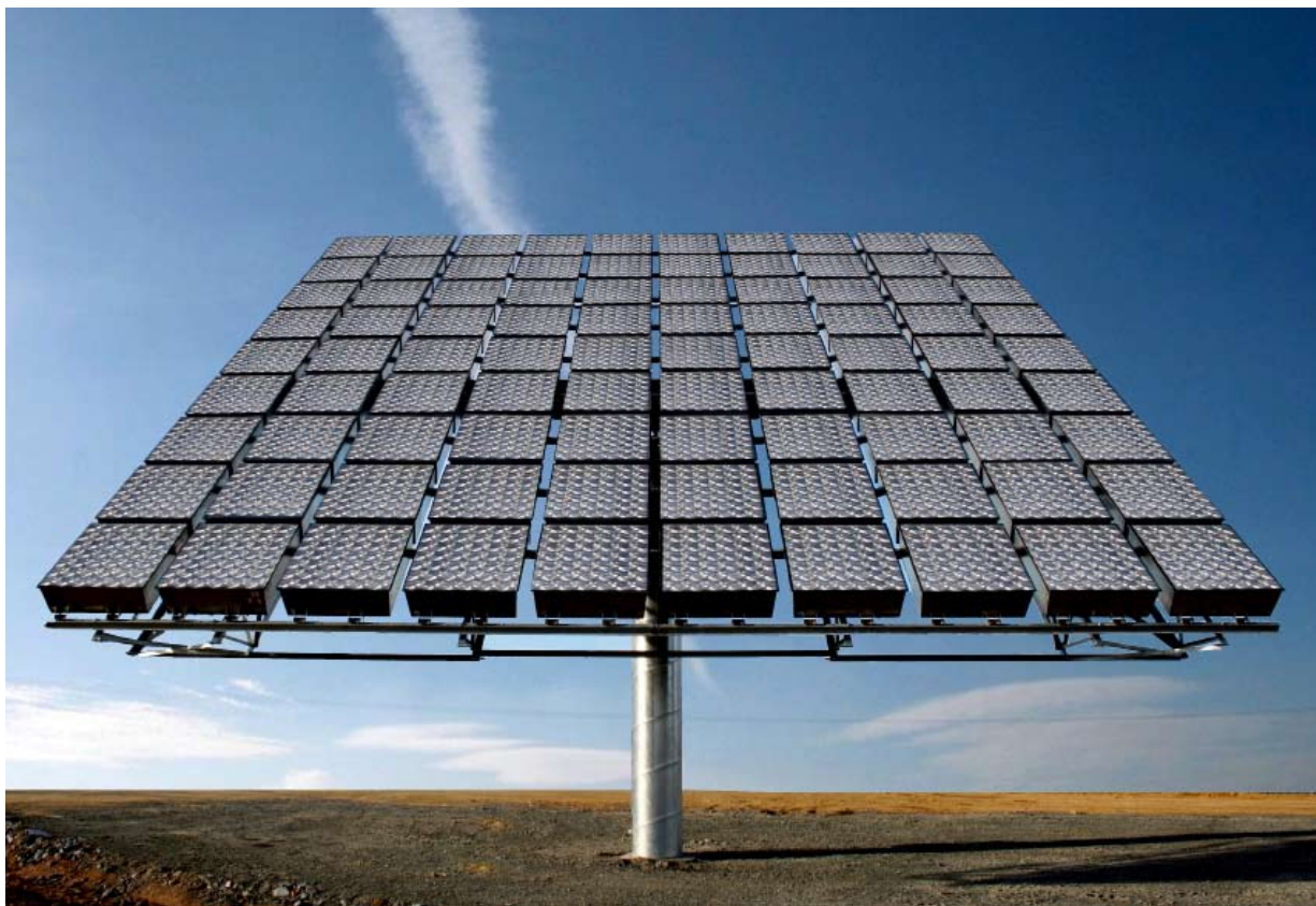
High-concentration photovoltaic (HCPV) module
