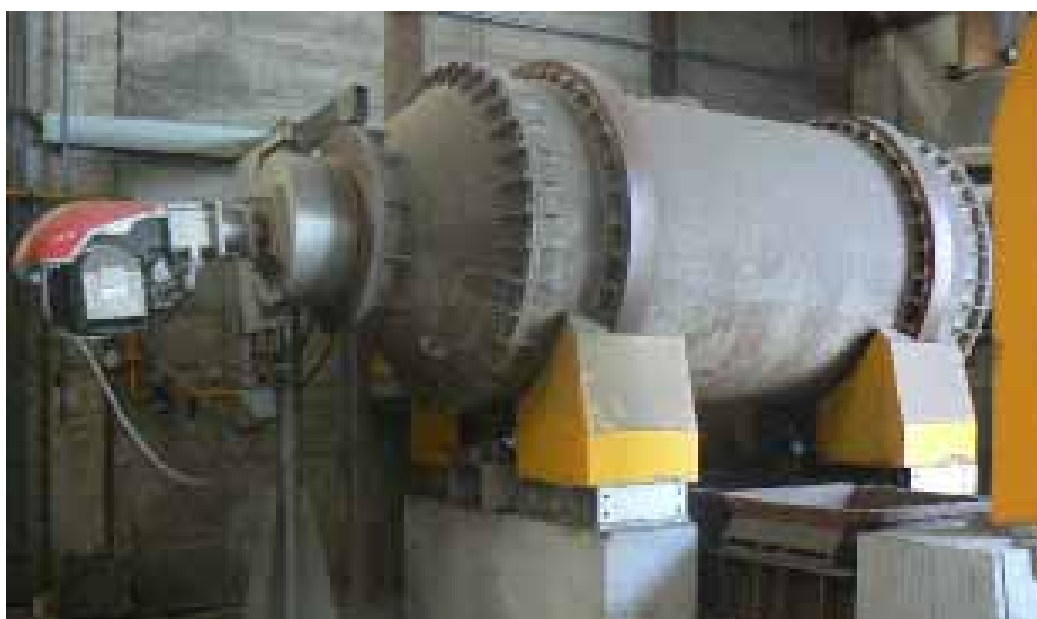
Rotary furnace with 1 t of capacity to be installed at Valladolid
