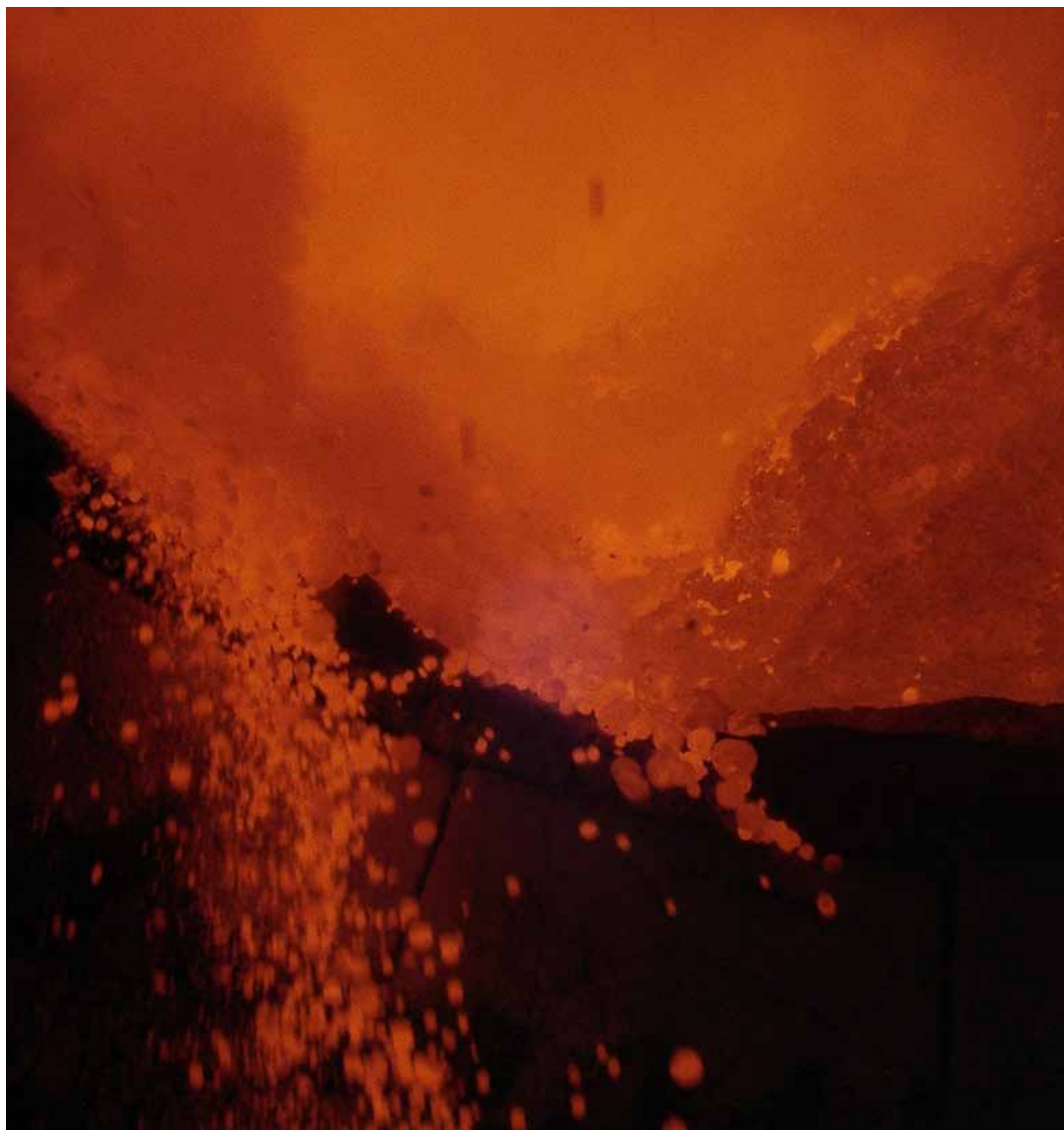
Slag falling from the Waelz furnace at Befesa Zinc Aser facilities, Spain
