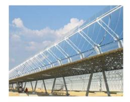
**Operating principle:** Parabolic troughs are used to track the sun and concentrate sunlight on to the thermally efficient receiver tubes placed in the trough focal line. In these tubes, a thermal transfer fluid is circulated, such as synthetic thermal oil. This oil is then pumped through a series of heat exchangers to produce steam. The steam is converted to electrical energy in a conventional steam turbine generator.
